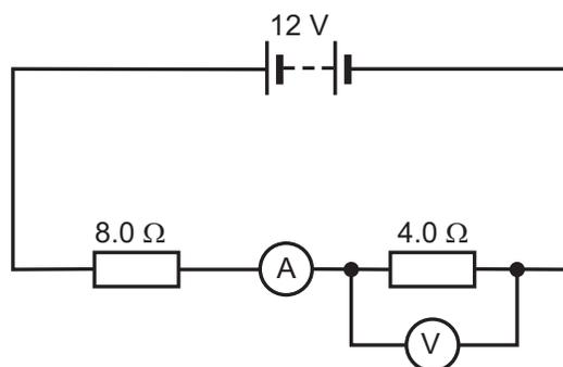
What are the readings on the ammeter and on the voltmeter, and how much charge passes through the 4.0 Ω resistor in 20 s?
